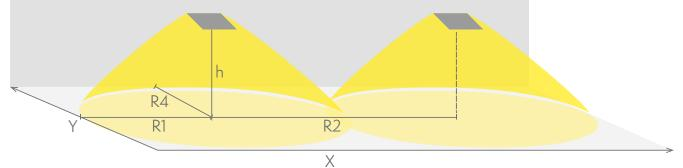
R1 distance from wall (X axis) R2 installation distance between lights (X axis) R4 distance from wall (Y axis) TWT9971W
