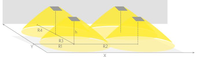
R1 distance from wall (X axis) R2 installation distance between lights (X axis) R3 installation distance between lights (Y axis) R4 distance from wall (Y axis) TWS6392WA
