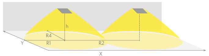
R1 distance from wall (X axis) R2 installation distance between lights (X axis) R4 distance from wall (Y axis) TWS6392WA
