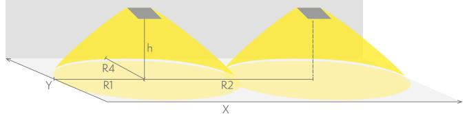
R1 distance from wall (X axis) R2 installation distance between lights (X axis) R4 distance from wall (Y axis) TWT9271W
