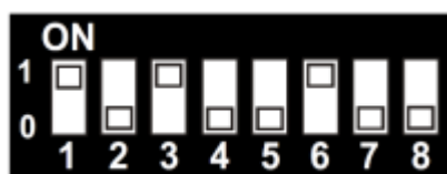
DIP-innstilling for Nortek Standard Tone og deaktivert flash
